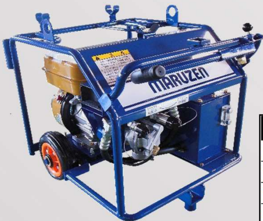
HYDRAULIC POWER UNIT MODEL UH070
