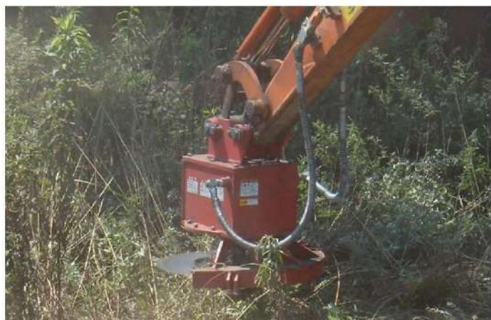
3. Blade for hard grass / bamboo Teeth : 100pcs
